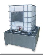
Galvanised Steel with Drain Plug Spill Capacity: 1100L Load Bearing Capacity: 2000kg Dimensions in cm (L x W x H): 136cm x 136cm x 70cm Weight: 160kg
